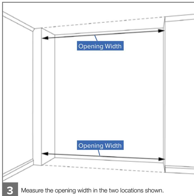
**These measurements will allow us to calculate the size of each door.**
