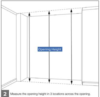
These measurements will allow us to calculate the size of each door.
